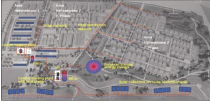
Figure 8: Site plan of the solar assisted district heating system in Crailsheim, Germany
