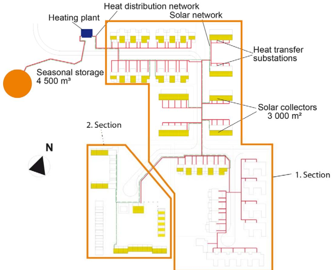
Fig. 2: Site plan of the CSHPSS in Hamburg-Bramfeld
